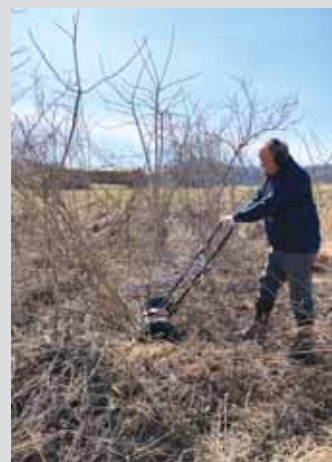
Path-Maker chews through small stems and saplings, cutting them at ground level.
