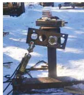
Head of the hydraulic wrench is a 12 by 36-in., 1-in. thick steel plate. Erdman drilled holes in all four corners of the plate and cut out a hole the size of the nut to be turned.
