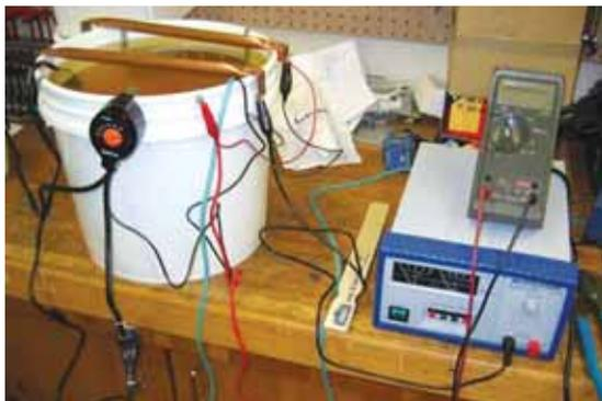
Electroplating tank and power source.
