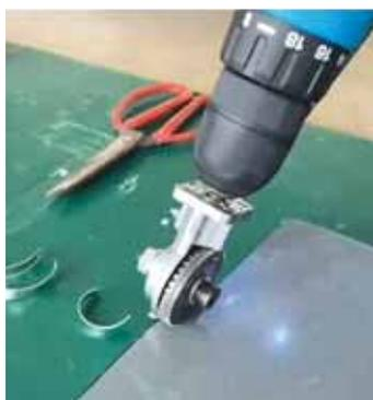
Made from high manganese gear steel, the drill shears are advertised as the perfect tool for car and house maintenance projects, including cutting metal roofs, HVAC vent pipes, and other forms of sheet metal.
