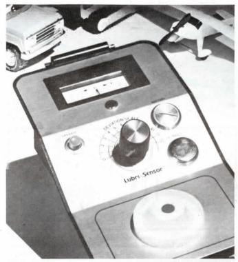
The Lubri-Sensor makes it possible to determine when oil is still usable, permitting longer intervals between oil changes. Provides advance warning of potential mechanical failure by detecting the presence of metal particles.
