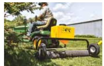
Liquid goes through the piping and streams down on the carpet. The wet carpet then rolls over and presses the chemical on the plants.
