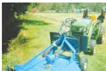
"I welded a quick attach plate with 3-pt. mounts to my loader's quick attach plate and added a hydraulic motor driven pto to it," says Zawalick.
