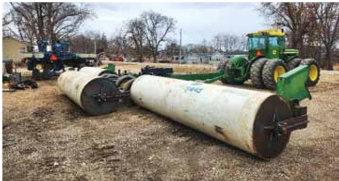
Farmer built a three-section 42-ft. wide field roller using the frame and wheels from a Deere 7000 16-row planter and three used anhydrous tanks.
