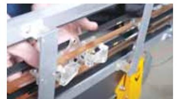
Thrower uses servo motors, double sided timing belts and an electromagnet to control knives.
