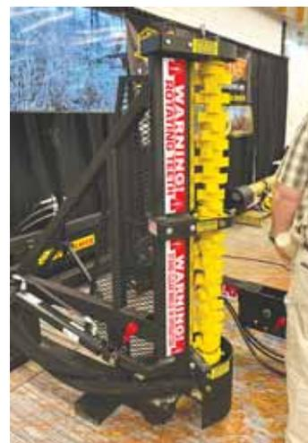
**Weighing only 265 lbs., the 48-in. Baby Beaver cuts through limbs and trees up to 3 in. in diameter at 4,500 rpm’s.**
