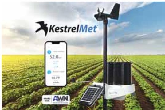
**Above ground, the KestrelMet 6000 weather station gathers information about rainfall, wind speed and direction, relative humidity, temperature, and barometric pressure.**
