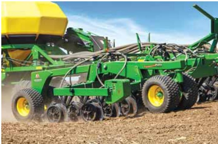
**Installation involves the removal of the factory-installed gauge wheels and beams from the frame. Once the TerrainFlex walking beam has been installed and the gauge wheels added, the air drill is ready to go.**
