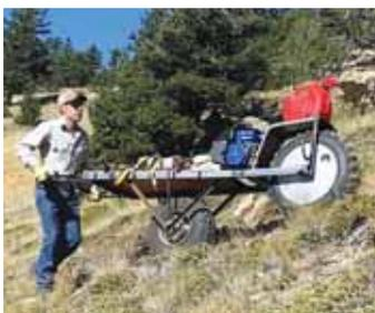
**MacLean's "contraption" is a cow path variation of a powered wheelbarrow using wheels from an old motorbike and quad.**
