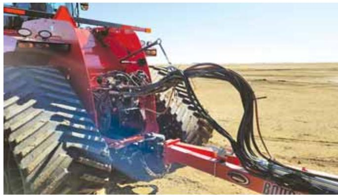
**Lend-A-Hand is a swinging arm mounted on the back of the tractor to keep hydraulic hoses and electrical lines out of the drawbar and PTO.**
