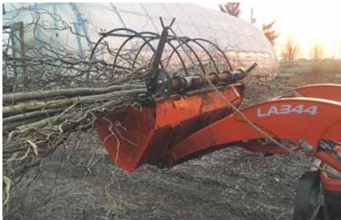
Currently, the tines fall 8 to 10 in. ahead of the bucket edge. Tschetter plans to add removable teeth to extend the bucket's reach.
