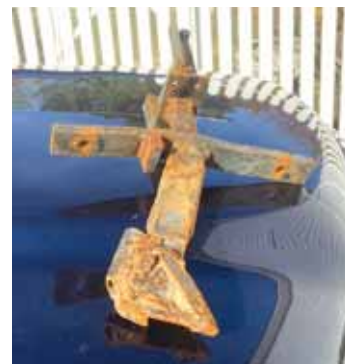
Gardner made a simple plow and welded a small pipe behind it for the wire to move through.
