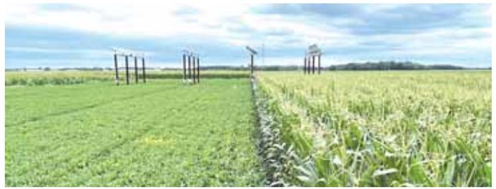
Arrays of solar panels were erected over corn fields to study the relationship between the sustainable generation of solar power and its impact on crop production.
