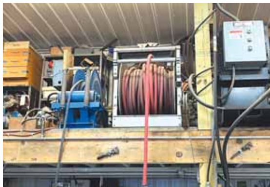
Bauer’s power reels are all mounted on the second level of his shop and have drop cords to operate them.
