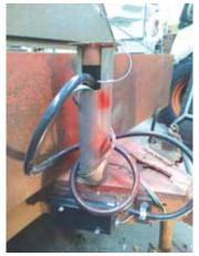
McLaen has an easy way to prevent trailer connections from getting drug and damaged. He stores them up and out of the way.
