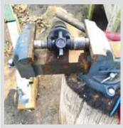
John Rochester, Charlotte, N.C.: "I've found that I can use sockets and a vice to remove a U-joint from the end of a driveshaft. I put one socket on the bearing cap and make the other one big enough for the cap to push through.
