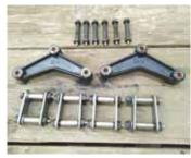
Another trailer sore spot with McLaen is car trailer suspension, in particular, the nylon bushings and hard-to-lubricate bolts at spring ends, shackles, and equalizers.
