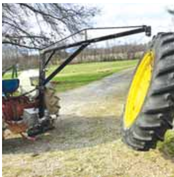
Thomas' 3-pt. crane lifts tractor tires without hydraulics.
