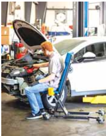
Ergo-RS creeper chair lies flat like a regular creeper, or the seat back can be locked at multiple angles.
