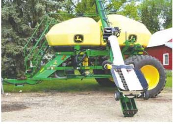
ACX-Retractor Kit doesn't telescope out. Instead, the 10-ft. extension sits on top of the cart's OEM auger until needed
