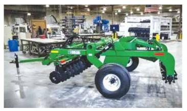
"You can lift it or lower it hydraulically on the fly depending on how much dirt you need to move. Combined with the aggressiveness of the disk angles, you can pull a little or a lot of soil to fill ruts," says Clifton.
