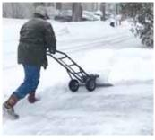
Plow attaches with a stainless-steel bar and two handles to the hand truck lift plate.
