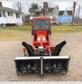
"I built a mounting bracket on the blowers to match the one on my tractor," McCallum says. "I just take off my quick attach bucket, drive up to the blowers, put in two pins, and plug in the power cord from the tractor."
