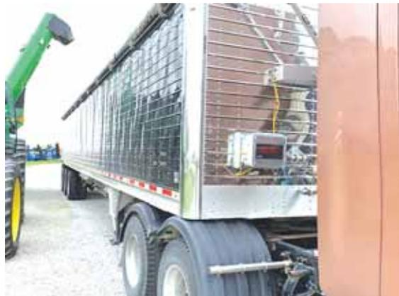
Whalen designed a system to measure the pressure change and calibrate it to the amount of grain in hopper bottom trailers.
