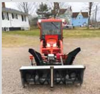
"I built a mounting bracket on the blowers to match the one on my tractor," McCallum says. "I just take off my quick attach bucket, drive up to the blowers, put in two pins, and plug in the power cord from the tractor."
