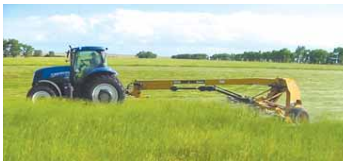
Transport is straightforward as the independent cutters hydraulically fold toward the hitch reducing the overall unit size to 9 ft. in width.
