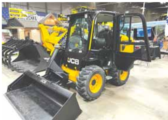
Skid steer cab is offset with a side access cab and a side boom.
