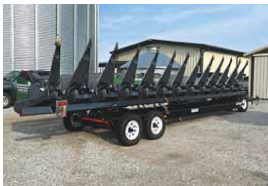
Mainero corn head has tungsten carbide self-sharpening opposing knife rolls that create an aggressive crimping action to cut and damage stalks so they easily decompose.
