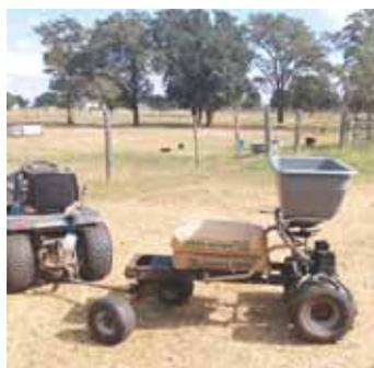
Sonsel’s spreader is made from an old garden tractor and a pull-behind spreader.
