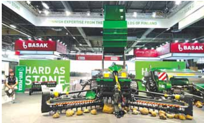
Stone collector uses pto to drive a pair of rakes on gauge wheels that run the opposite of ground direction in a 'V' pattern, extending on either side of the center tines and bucket.
