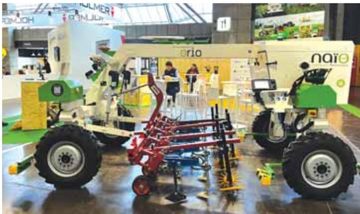
Orio robot features a series of ground shovels, packer wheels, and rotating fingers and is driven by four 3000-watt 48-volt electrical engines powered by four rechargeable lithium-ion batteries.
