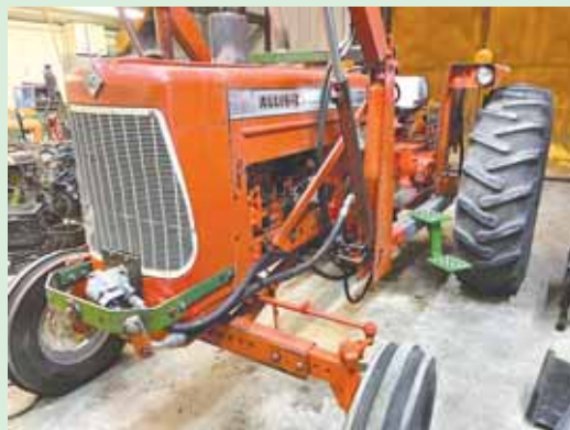
Robert Bauer installed a 17-gpm hydraulic pump on the front of his D-19 Allis to provide continuous oil flow for his mounted loader. Controls are located to the left and below the tractor seat.
