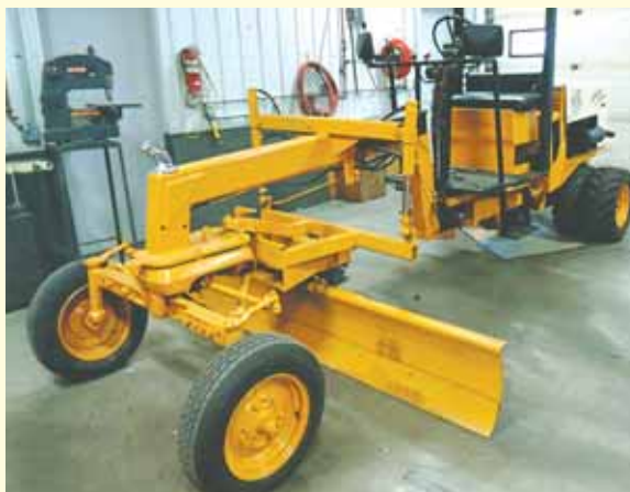
Adelman used an 80's Ditch Witch as the base for his grader with an 8-ft. blade.
