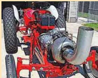
Frame and hood had to be extended 9 1/2 in. for the turbine and transmission.
