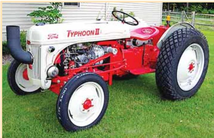
Baumann's Typhoon II is outfitted with a 40-hp. turbine and hydrostatic transmission.
