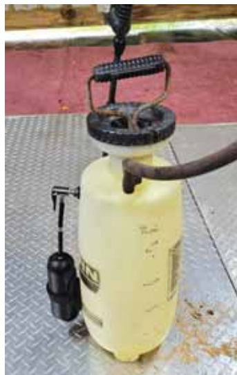
Smith converted an old hand sprayer to use a small battery-powered pump.
