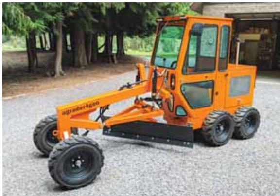
"I ended up using Toro zero-turn lawn mower individual trans-axles so I could spread the frame a bit and made some linkage to tie the two drive motors together," Hadler says.
