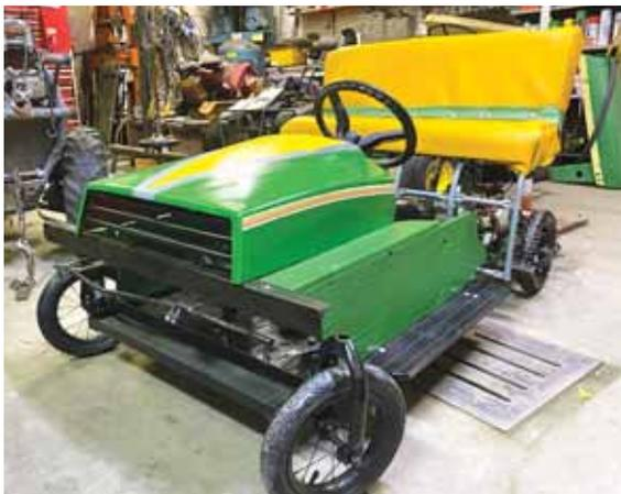
Heron's original plan was to build a smaller cart, but he decided to expand it to add a longer steering shaft. He installed an old 70 cc Honda clone, electric-start engine from a scrapped quad to power the runabout.
