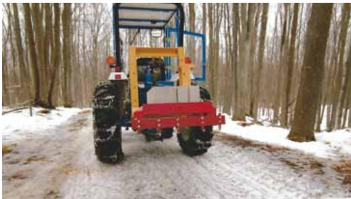
Two 3/8-in. bolts secure the ice gouger's angle iron frame to the carry-all, so it's easy to put on and take off.
