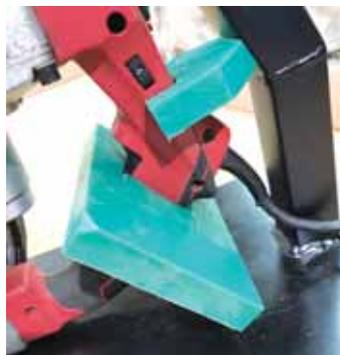
High-density polyethylene holding the trigger in the on position.
