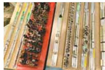
Tilley mounted socket rails to the top of a safe deposit box to keep his tools organized.
