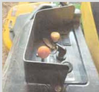
Garnet Powers, Marsden, Sask.: "After breaking two keys off and bending the choke cable while mowing around trees, I installed a shield around the engine controls on my zero-turn mower. Now those low branches just slide up and over the top, doing no damage."
