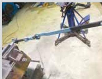
Tim Barndon Jr., Kulin West, Australia: "I made an extension bar for box end wrenches. It has tabs that wrap around the wrench so it's much safer to use than a pipe or other methods. No more skinned knuckles or slips."
