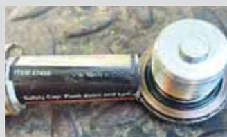
Gerald Rippes, San Antonio, Texas: "I attach magnets to the inside of oil pan drain plugs on equipment. I buy rare earth magnets from Harbor Freight at \$3 for 10 magnets. Works great to pull metal filings out of the oil. Each time I pull the plug, I clean off the magnet."
