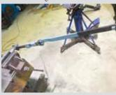
Tim Barndon Jr., Kulin West, Australia: "I made an extension bar for box end wrenches. It has tabs that wrap around the wrench so it's much safer to use than a pipe or other methods. No more skinned knuckles or slips."
