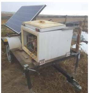
Portable water pump showing solar panel and batteries inside old chest freezer turned on its side.
