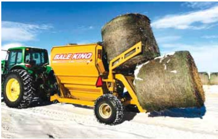
Loading forks lift one bale into the tub. They raise a second bale into position directly behind the tub for the grapple arms that are added with the kit. The loading forks then lift a third bale to a transit position.
