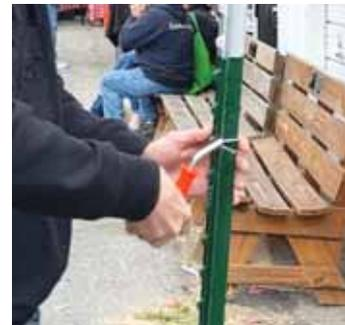
Show-Me Twister tool secures T-post fence clips on wire fences.
