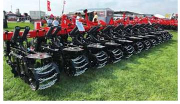
The 1210's uniquely designed row units consist of adjustable 25-in., 6-ga. cutting coulters and scrapers, 16-in. floating notched disc blades to clear residue from the strip, adjustable depth shanks, and Kuhn's exclusive Strik'R technology chain reels.
