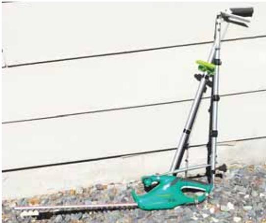
**Bohl bent 3/4-in. light wall conduit and bolted it to a bracket on the top of the trimmer and flattened one end of the conduit to fit under the trimmer.**
