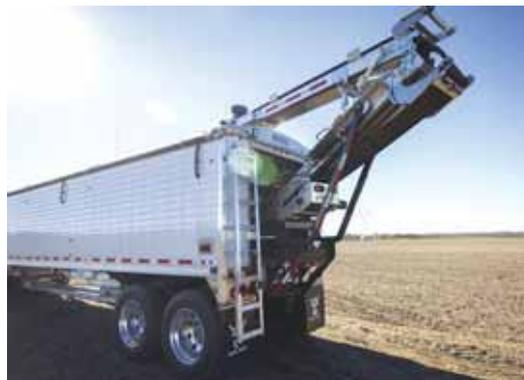
**Rear delivery chute features over 10 ft. of horizontal swing, making it easy to position receiving equipment. The spout offers 16-ft. of clearance allowing filling at a more ideal angle.**
