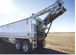
Rear delivery chute features over 10 ft. of horizontal swing, making it easy to position receiving equipment. The spout offers 16ft. of clearance allowing filling at a more ideal angle.
