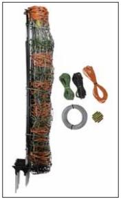
Posi/Neg netting has alternating electrified (orange) and non-electrified (green ground) strands. Animals are shocked when they make contact with both strands.
