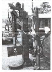
cylinder. What's more, I mounted a hydraulic-powered cable winch fitted with a pair of log tongs on top of the big splitter mast so I can drag big chunks of wood onto the splitting table without any lifting.
