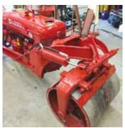
Original worm gear and steering was replaced with a hydraulic cylinder.
