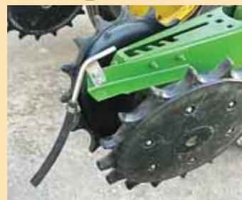
Side view of tubes and brackets before adding feeder line to pump.
