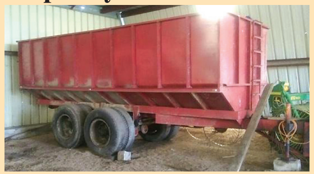
William Davis used the running gear from an old tandem axle semi trailer to build this 500-bu. rear-unloading grain hauler.
