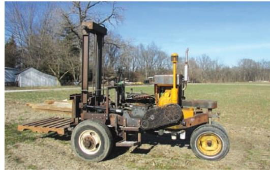
He started with the rear end and frame off a 1970's Chevy 1-ton dually pickup, turning the frame backward so the rear axle and wheels are up front.
