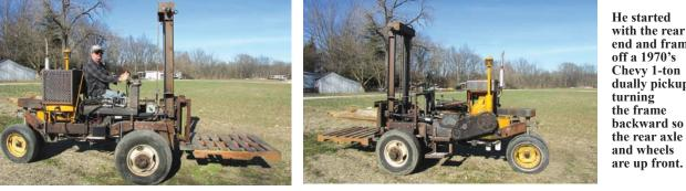
end and frame off a 1970's Chevy 1-ton dually pickup. turning the frame backward so the rear axle and wheels are up front.
