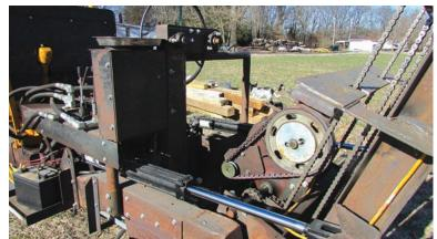
The motor and gearbox off a David Bradlev walk-behind tractor is used to chain-drive the forks up or down.
