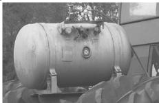
Propane Enhancer injects a little propane into diesel engines for faster speeds, more power, and a cleaner burn in tractors and trucks.
