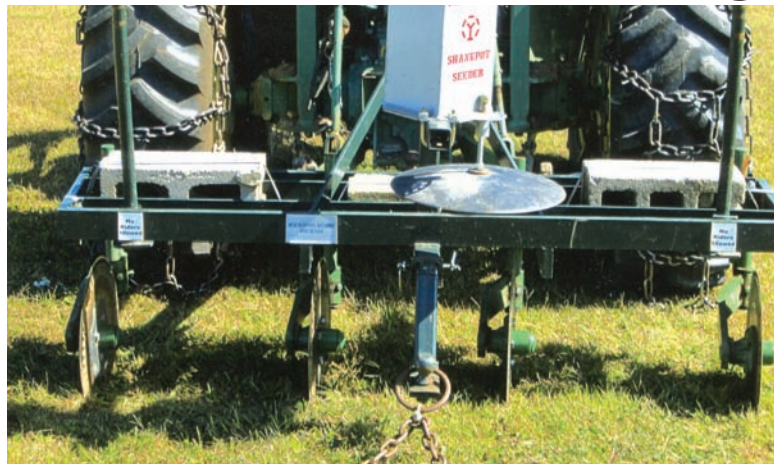
BRO pasture aerator uses 4 wavy coulters and a Shankpot Seeder for one-pass aeration and reseeding.
