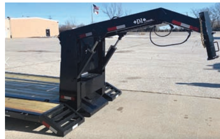
Trailer’s gooseneck hitch releases front of trailer bed onto the ground for loading and unloading.
