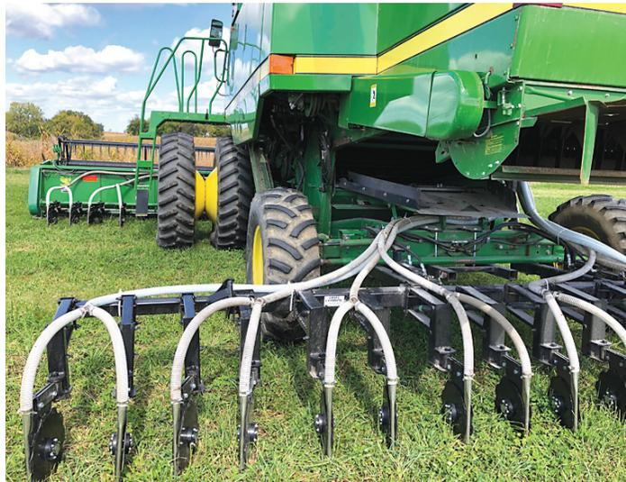
A 15-ft. toolbar with single disc coulters mounts on combine’s rear axle, with 6-ft. toolbars mounted to each end of the 30-ft. soybean header.
