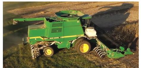
A 30 cu. ft. Montag seed tank mounts above the header on the right side.
