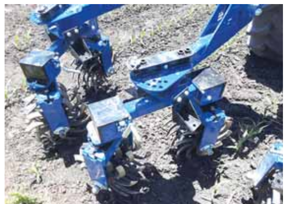
Swinging Spider allows for easy adjustments of the arm and the individual “spiders”.
