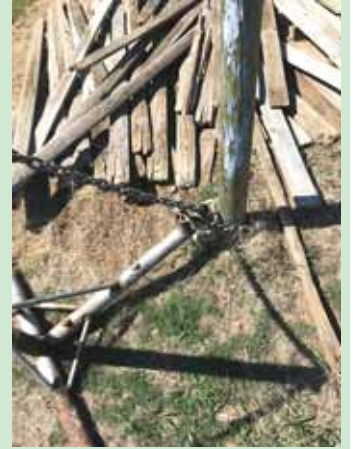
The pivot pipe on the ground acts like the claw of a hammer to pull out fence posts.
