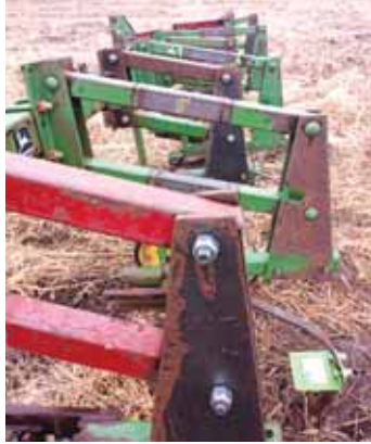
Curt Forde added an 8 in. extension to the shank mounts on every other row of his cultivator to create a staggered soil flow off the shovel.
