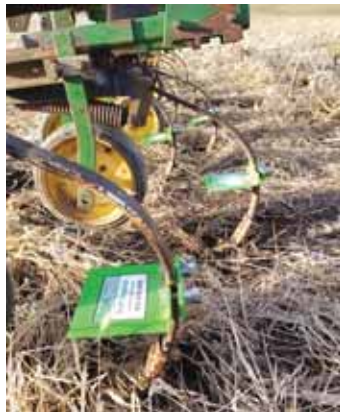
Flowshields mounted on each shank divert soil down and over grass and oats around the growing crop.
