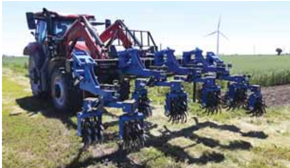
Rotary hoe allows control of the angle and down pressure for better weed control.
