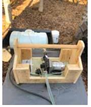
Carry box made to hold and secure a pump used for moving Maple sap to a holding tank.
