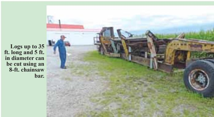
Logs up to 35 ft. long and 5 ft. in diameter can be cut using an 8-ft. chainsaw bar.
