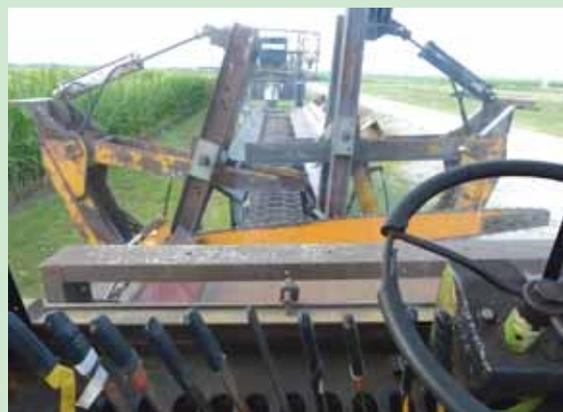
Most of Ewen's firewood processor came from a crane built to lift modular homes.
